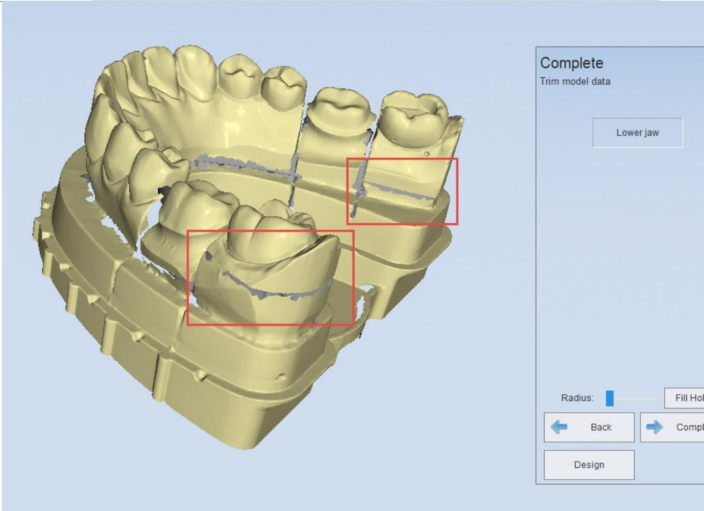
Rotate the jaw to observe that there are parting line between the aligned tooth and jaw, shown as the figure below.
