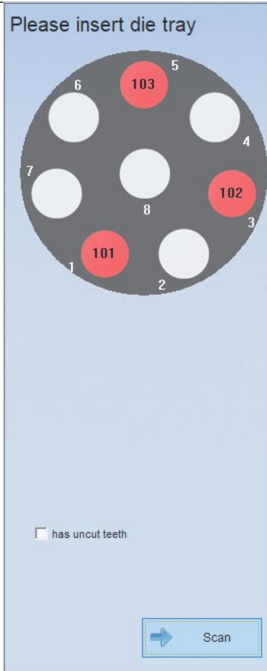
Make sure that die tray are inserted with die before you click "Next" to start scanning. After scanning, you can "Add scan" to get better scan result. Then click "Apply" to optimize the scan data as below.
