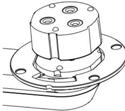
**Static articulator scan pad:** use it during static bite scan. See Artex articulator below as an example:
