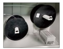
Filament dry room have 2 temperature options to set. (45 degree /65 degree.) Note: The PLA,PVA,HIP filaments are disable the drying function of the consumables bin.
