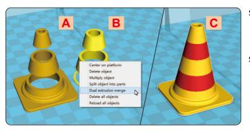
Step 1: Load 2 models you want as shown in figure [A] and [B].
