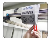
Step 1: loose the screws on the back.
